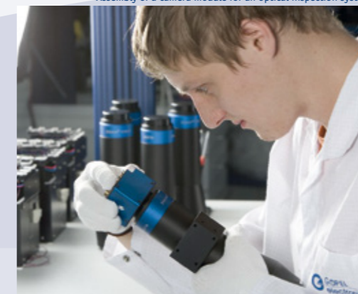
© GÖPEL electronic GmbH: Assembly of a camera module for an optical inspection system
